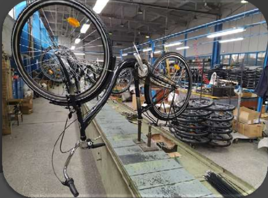
- Assembly line conveyer type (two lines) feed by Wheel building robots
